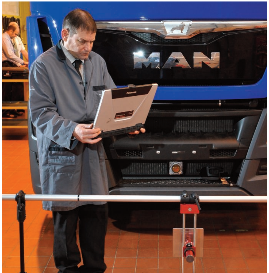
Checking AEBS and ACC radar sensor set-up with the laser-based tracking gauge
